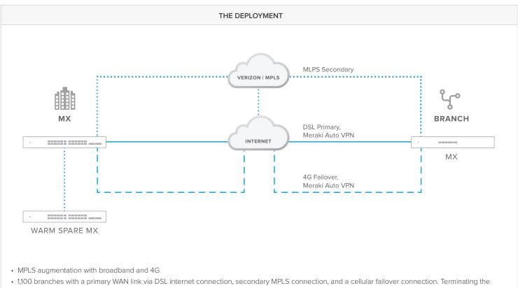
tunnels at headquarters are two Meraki MX600s in warm spare configuration preventing a single point of failure.
